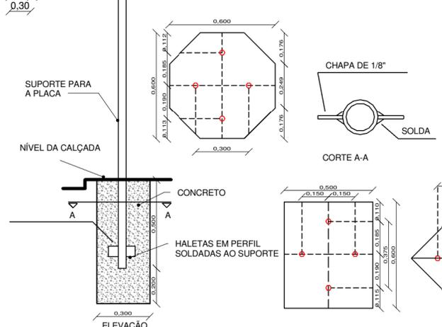
**JOSE ALDO DETALHES DE PLACAS, DETALHES CONSTRUTIVOS**
